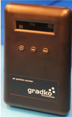
**Description:** Laser particle counter for counting individual particles. Sizing bands of small and large, according to calibration.
