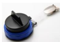
1. Apply sample identifier in oblong space at back of the sampler.
