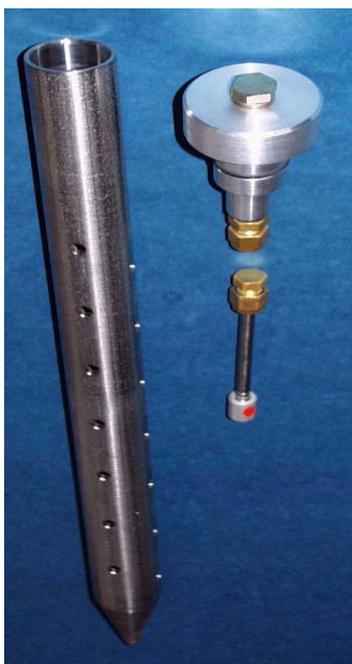
Concentrations absorbed by the tube are measured by thermal desorption and analysis by Gas Chromatography / FID or Mass Spectroscopy (UKAS Accredited Methods).
