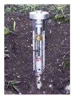
7. Push the assembled Soil Probe cap unit into the Soil Probe. The unit is now ready for sampling (sampling period of 1-4 weeks). Mark or record the location of the Soil Probe for easy identification at the end of sampling.
