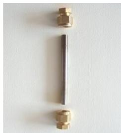
1. Use Tubelock tool to remove both brass end caps from the VOC tube.
