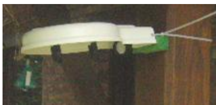
Figure 3: Dedicated shelter for the Gradko sampler
