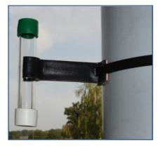
**Description:** Acrylic tube fitted with a green and white thermoplastic rubber caps. The green cap contains the absorbent and the white cap is fitted with a filter to prevent the ingress of particulates. This tube is designed to simultaneously passively monitor gaseous  $NO_2$  and  $SO_2$ . Analysis of exposed tubes is carried out by Ion Chromatography (UKAS Accredited Methods).
