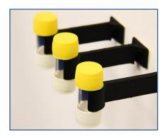
**Description:** Fluorinated ethylene polymer tube fitted with yellow and white thermoplastic rubber caps. The yellow cap contains the absorbent. A one-micron porosity filter is fitted to the white cap to prevent the ingress of airborne particulates containing ammonium ions.
