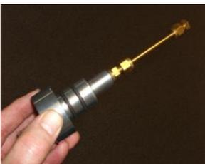
5. Slide the VOC Tube into the Soil Probe cap unit and tighten using Tubelock tools. The nut should be finger-tight and then turned  $\frac{1}{4}$  turn ONLY with the Tubelock tool. **DO NOT OVER TIGHTEN, DO NOT USE SPANNERS.** Tightness of the tube can be checked by gently pulling it to ensure that it does not slide out.
