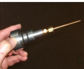
6. Remove the remaining brass end cap from the GROOVED end of the VOC Tube.
