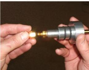
4. Using Tubelock tool, unscrew the lower brass nut cap from the Soil Probe cap unit, until it is loose enough to slide the VOC Tube into.
