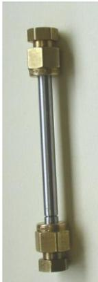
11. Remove the Soil Probe cap unit from the Soil Probe. Refit the brass end cap with the coloured spot to the open end of the VOC Tube. Caps should be finger-tight and then turned ¼ turn ONLY with the Tubelock tool. **DO NOT OVER TIGHTEN, DO NOT USE SPANNERS.**
