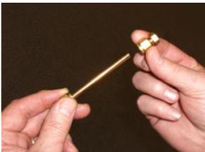
3. Remove the brass end cap from the NON-GROOVED end of the VOC Tube using the Tubelock tool.
