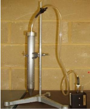
7. Push the assembled Soil Probe cap unit into the Soil Probe. The unit is now ready for sampling.
