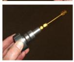
5. Slide the VOC Tube into the Soil Probe cap unit and tighten using Tubelock tools. The nut should be finger-tight and then turned ¼ turn ONLY with the Tubelock tool. DO NOT OVER TIGHTEN, DO NOT USE SPANNERS. Tightness of the tube can be checked by gently pulling it to ensure that it does not slide out.
