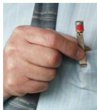
3. Push the diffuser cap on the open end of the tube.
