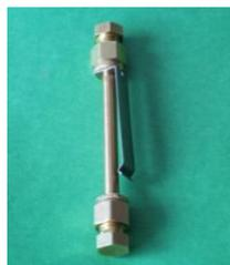
5. After exposing the tube for the required period of time, remove the diffuser cap. Use the Tubelock tool to place the brass end cap on to the tube. **DO NOT OVER TIGHTEN, DO NOT USE SPANNERS.** Test the tightness of the caps by gently pulling them.
