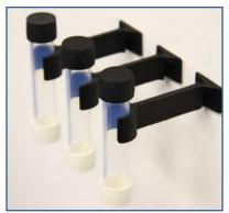
**Description:** Fluorinated ethylene polymer tube fitted with black and white thermoplastic rubber caps. The coloured cap contains the absorbent. A one-micron porosity filter is fitted to the white cap to prevent the ingress of airborne particulate nitrate.
