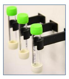
**Description:** Acrylic tube fitted with green and white thermoplastic rubber caps. The coloured cap contains the absorbent. A one-micron porosity filter is fitted to prevent particulate ingression.
